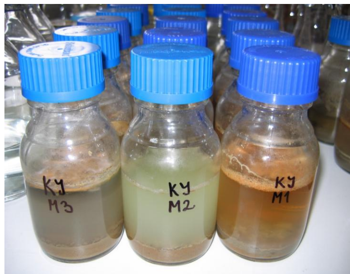
FIG. 7. THE FORMATION OF BROWN FINE GRAINED FRACTION OF IRON PRECIPITATE AFTER 19 DAYS OF THE SEDIMENT BIOLEACHING
