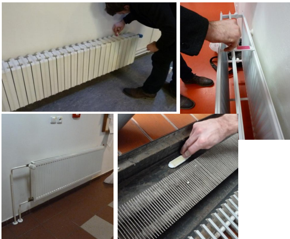
FIG. 3: POSITIONS OF SAMPLINGS ON THE TESTED HEATER
