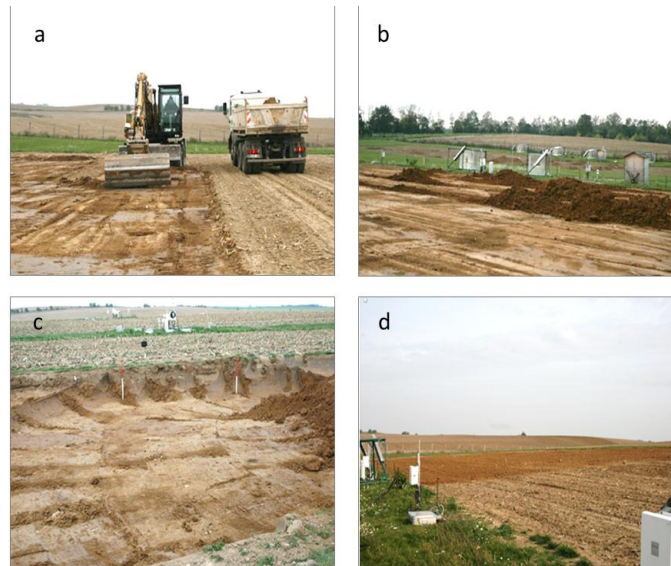
FIGURE 2. MANIPULATION PROCEDURE (OCTOBER 2010): (A) REMOVAL OF 6 CM AP AT PLOT 11, (B) ADDITION OF THE AP MATERIAL FROM PLOT 11 TO PLOT 10, (C) EXCAVATION OF BT (NEARBY PLOT 1), (D) SOIL SURFACE OF PLOT 11 AFTER HOMOGENIZATION.
