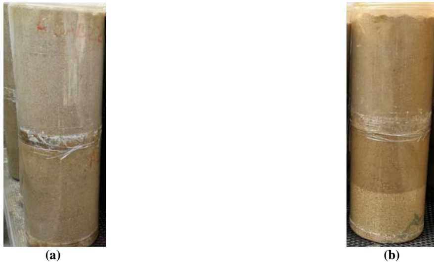
FIGURE 2: Appearance of the two types of tube used a) without filter b) with beach sand filter.
