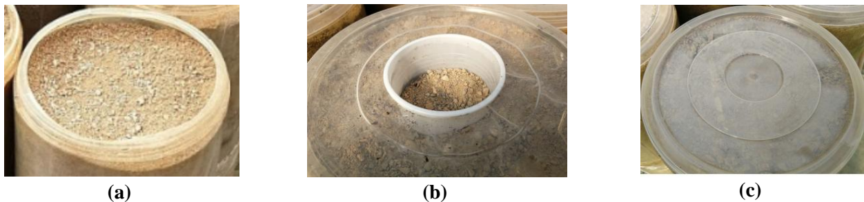
FIGURE 3: a) tube without surface protection b) tube with partial surface protection c) tube with full surface protection.
