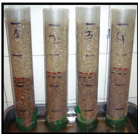
**FIGURE 5. Behaviour of specimens with sandstone after four days in contact with seawater**
