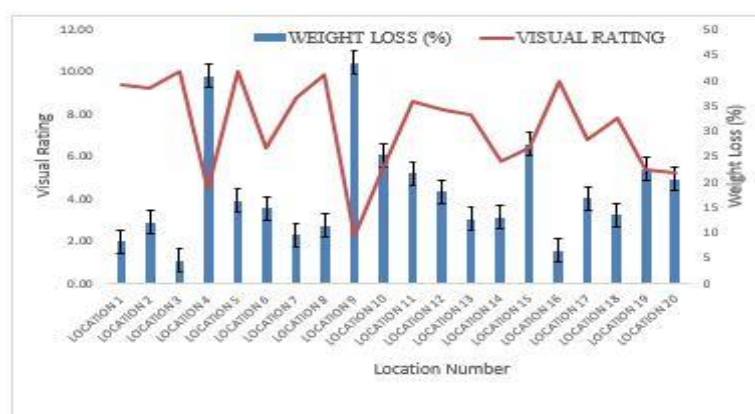
FIGURE 9: Severity of termite activities across the 20 locations within the AAUA campus as measured by the gravimetric weight loss and the ASTM D3345-17 visual rating.
