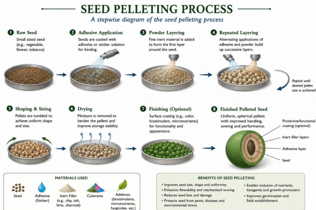
FIGURE 1: Schematic diagram of the seed pelleting process showing steps from raw seed to pelleted seed Note: The seed pelleting process typically involves: (1) Seed cleaning and sorting, (2) Application of adhesive/binder (e.g., gum arabica, maida gum), (3) Addition of filler material (clay, diatomaceous earth, etc.), (4) Addition of active ingredients (micronutrients, biofertilizers, pesticides), (5) Drying, (6) Sieving and quality control, (7) Packaging and storage.
