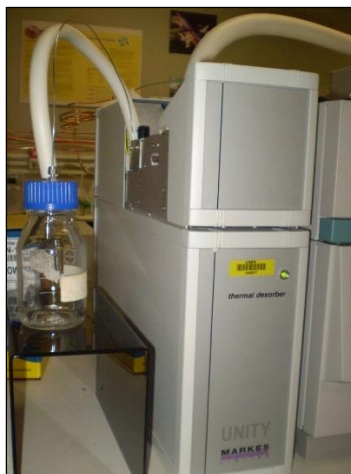
FIGURE 1: Dynamic headspace sampler attached thermal desorption unit
