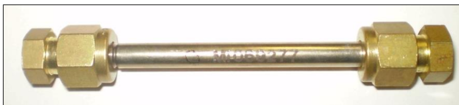
FIGURE 2: Example of sorbent tube, Tenax TA
