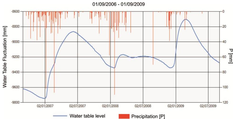
**FIG. 8 WATER TABLE DEPTH VS. PRECIPITATION**
