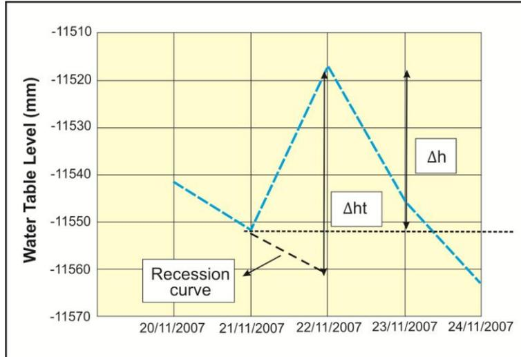
**FIG. 6 MEASUREMENTS TO BE PERFORMED FOR THE RECHARGE ESTIMATION**
