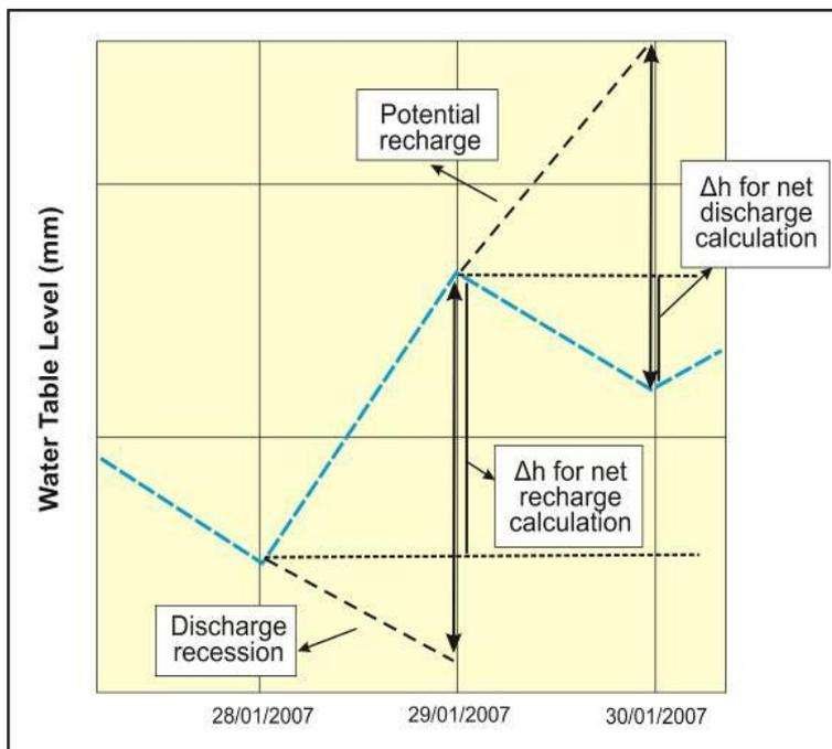
**FIG. 7 MEASUREMENTS TO BE PERFORMED FOR THE DISCHARGE ESTIMATION**
