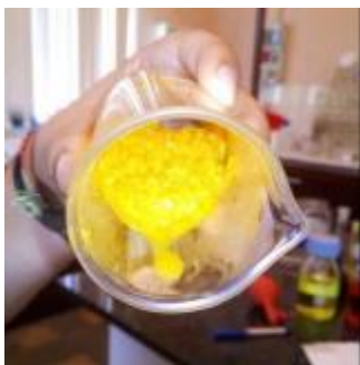
FIGURE 1: Detachment of a drop of liquid from the water-saturated solid
