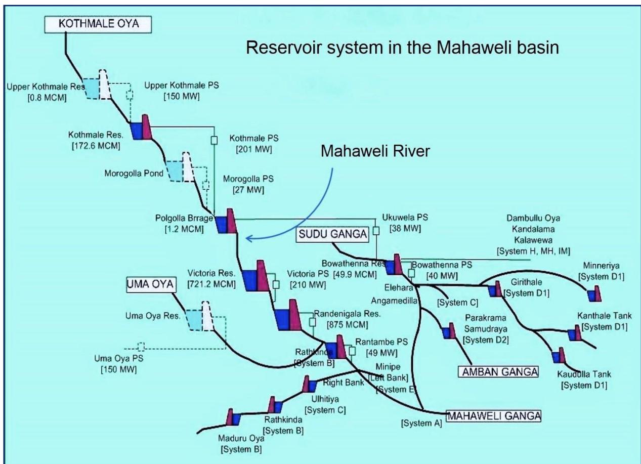
**FIGURE 1: CASCADE OF LARGE RESERVOIRS IN SRI LANKA SUPPLIED BY THE MAHAWELI RIVER**
