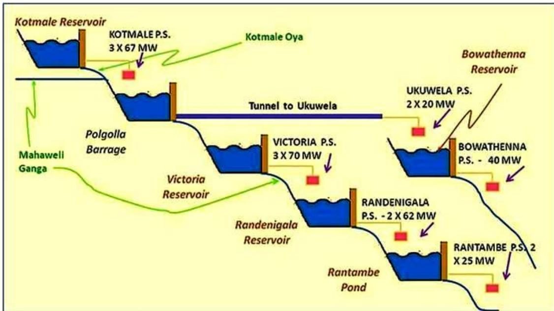
**FIGURE 2: CASCADE OF RESERVOIRS CONSTRUCTED IN THE RECENT PAST FOR THE GENERATION OF HYDROELECTRICITY BY TAPPING THE UPPER CATCHMENT REGION OF THE MAHAWELI RIVER IN SRI LANKA**
