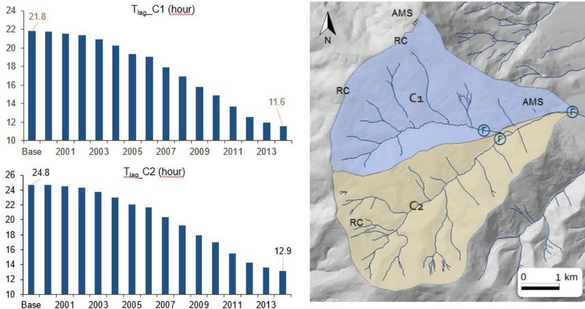
**FIG. 7. THE CHANGES OF THE SPEED OF WATER RUNOFF TLAG(HOURS) IN THE FOREST CREEK BY SUB-WATERSHED**
