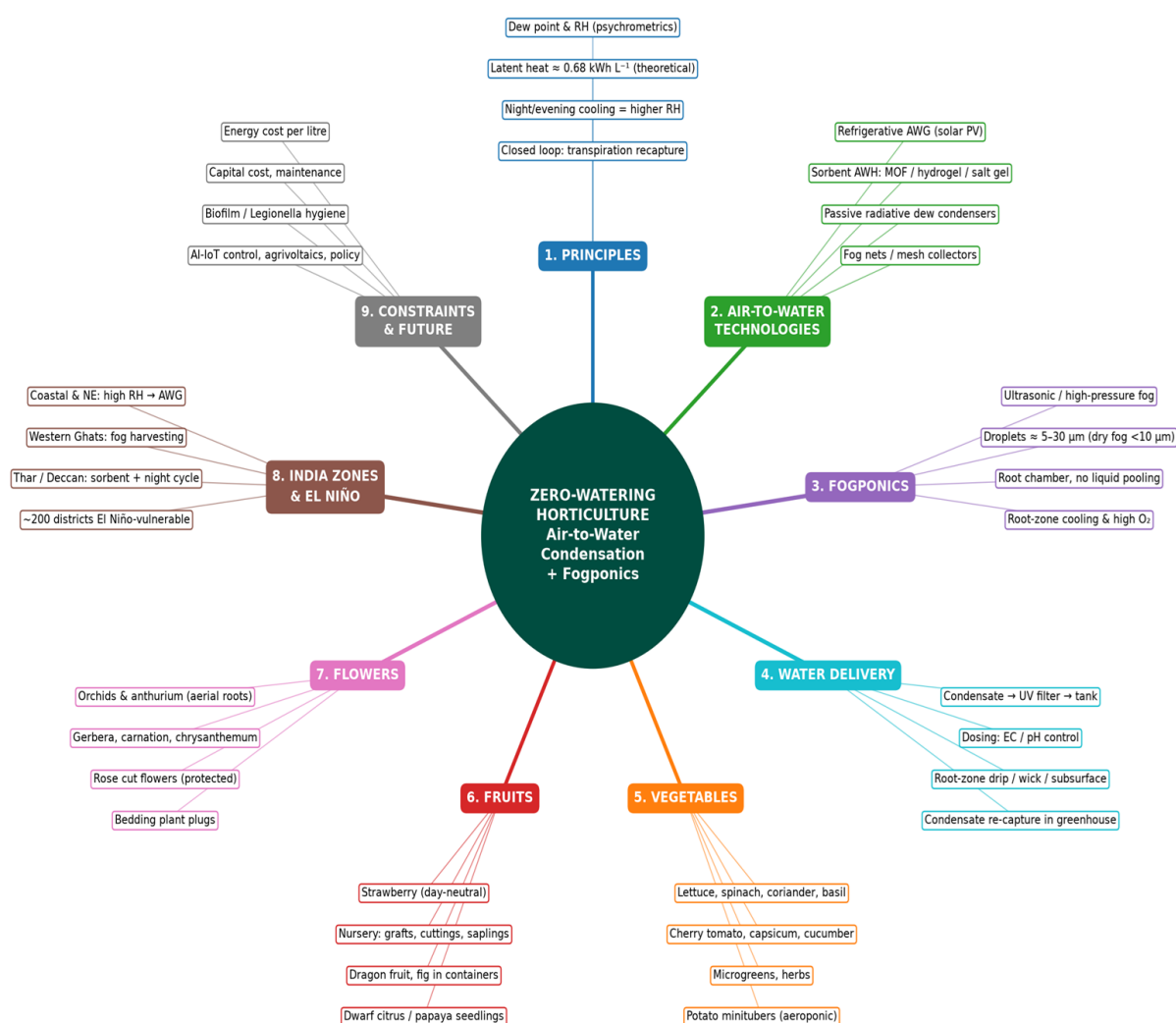
FIGURE 1: Mind map of zero-watering horticulture based on air-to-water condensation farming and fogponics, covering principles, technologies, delivery, crop groups, Indian agro-climatic zones and constraints.
