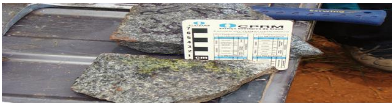
FIGURE 2: Samples of diabase from Taiano (municipality of Alto Alegre) with strong positive phosphomolybdate test.
