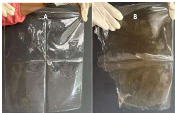
FIGURE 1: Images of fabricated (A) PVA–ninhydrin and (B) PVA–nano ZnO–ninhydrin composite films
