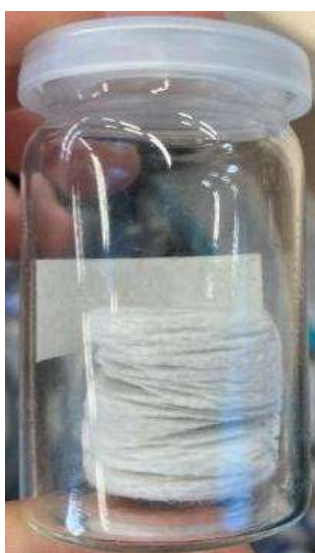
FIGURE 2: Control wipe (strip) with reagent and closed in an environment without any oxidizing agent, after one month (Own elaboration)
