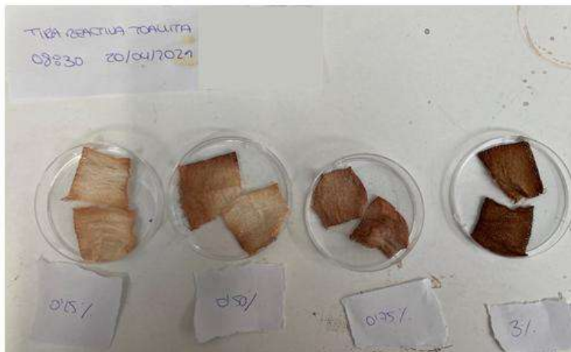
FIGURE 1: Reactive wipe (strip) with different concentrations of peroxide (Own elaboration)
