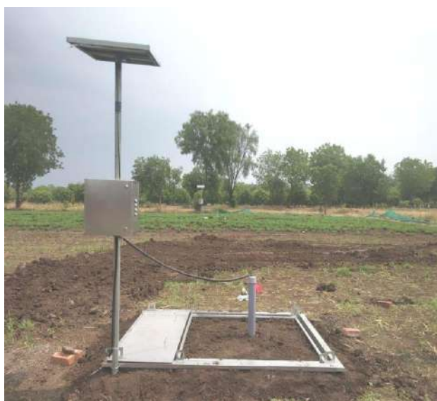
FIGURE 1: Technical Specifications of Weighing Type Digital Lysimeter
